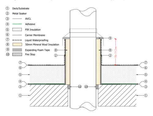
NOTE: The cravat termination needs to be applied immediately after the completion of the liquid applied membrane to reduce the risk of water ingress into the roofing system. Please note that this may not fall into the remit of the roofing contractor, therefore responsibility of this application needs to be determined prior to works commencing.
