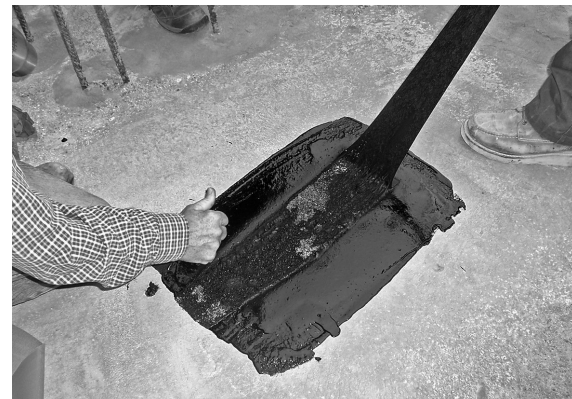
Figure Y – Cohesive failure (pass)
