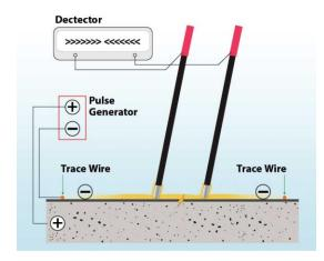
For this, a test area is set up by means of a loop of conductor wire. The enclosed section is thoroughly wetted, creating an electric "plate", which is insulated from the deck by the membrane system. The conductor loop masks extraneous signals from outside the area and can be wound around any earthed items within it (such as outlets, plinths, etc.).
