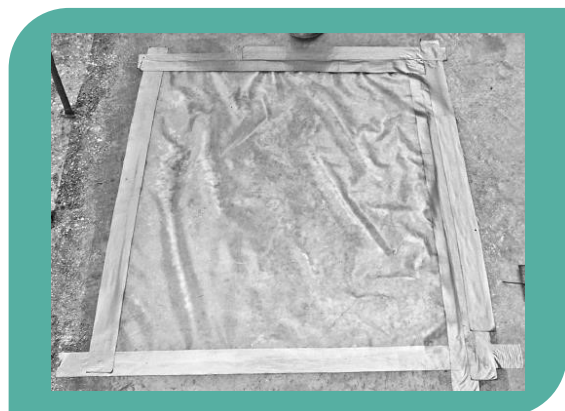
Figure 1 - Plastic sheet method
