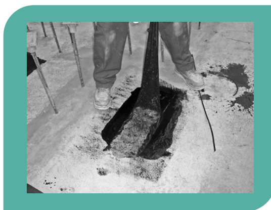
Figure 3 - Cohesive failure (pass)
