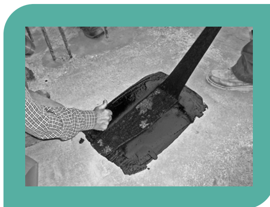
Figure 3 - Cohesive failure (pass)
